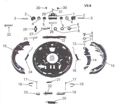
Lo and behold, I found that the '53 - '62 Chevy cars are the same. The later years have a minor change in the bolt assembly (Part #9 in Illustration #1). The early style used a bolt and nut, later it was changed to a pin with a snap ring.
