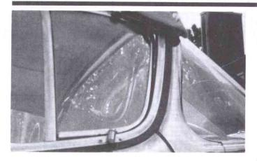
1953-1955 side windows came with the lower rubber water seal cloth covered, only at the front area. Black, or some say gray, material stopped at the lower ventilator support. The reason was to reduce squeaking while driving, caused by the vibration of the door against the window post.
