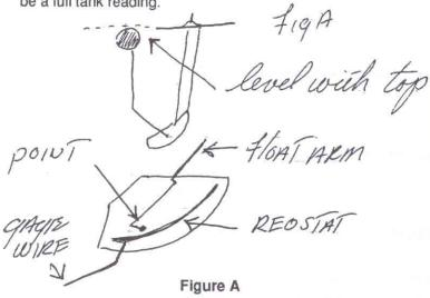
Comments: As the float point rides up and down on the reostat, a resistance is sent back to the gauge indicating gas level. It basically works the same as a temperature sender does (I wrote about that in Volume 2, Number 2).
