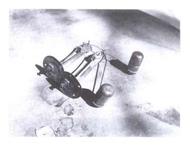
'53-'54-'55 fuel sender on right is for the Corvette. On the left is the '53-'54 pick-up truck sender, which is the same as the Corvette.
