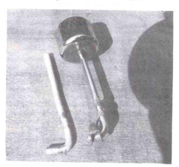
The button and rod for the soft top lid assembly differed from 1953 - 1957 and 1958 - 1962.
