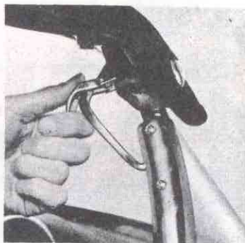
Fig. 44—Locking Top to Windshield Frame
