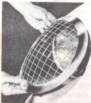
Fig. 75—Removing Rim, Screen and Housing
