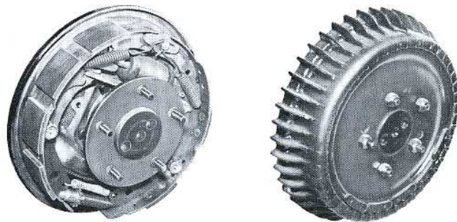
Deep finned cast iron drums and segmented ceramic-metallic linings offer virtually fade-free braking for the most competitive events.
