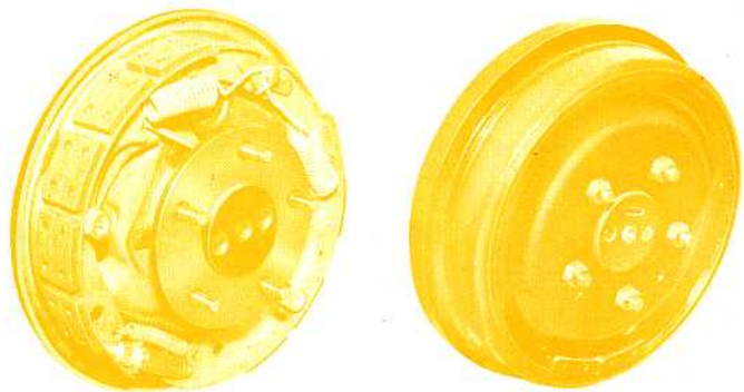
R.P.O. 686 segmented sintered-metallic linings and special finish brake drum. Shoes and drums are same width as standard brakes. Metallic linings are virtually unaffected by moisture.
