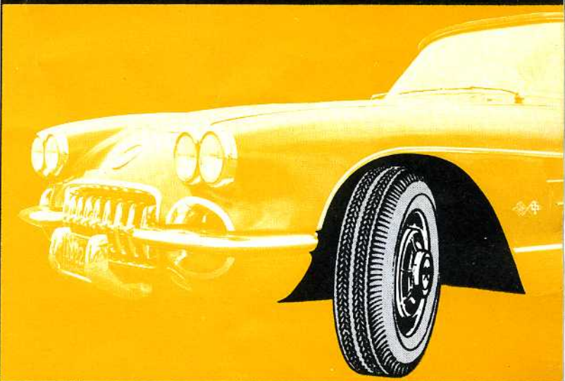
Optional nylon cord tire (L.P.O. 1408) installed on optional wide-base 15 x 5.50 K wheel (R.P.O. 276).
