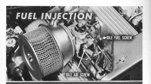
Correct idling of fuel injection engines is accomplished with the idle air and idle fuel screws. Initial setting of both is two turns open.
