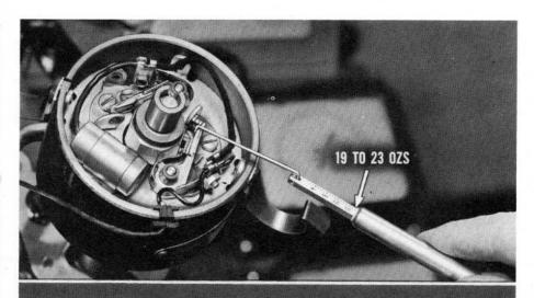
Check the breaker arm spring tension of each set of points with cam follower between lobes of cam. Tension range is 19 to 23 ounces. If more or less, adjust as follows—
